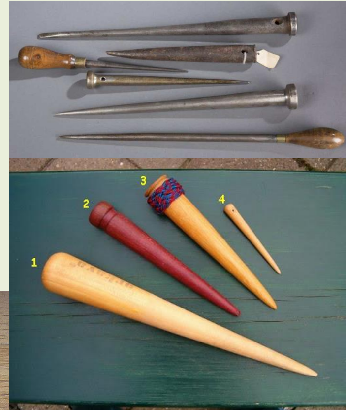
Tarred Marlin cord, Marlin spikes and Fids. [Marlin spikes and Fids are used to separate the strands of rope]
